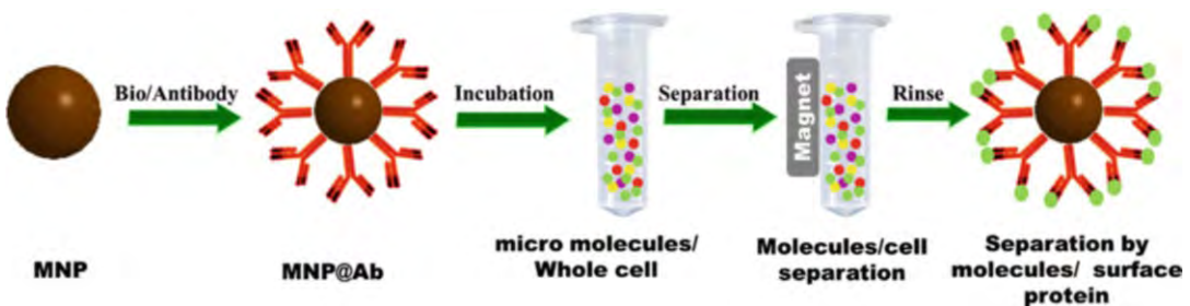
Fig. 8 Separation of a target protein antibody-conjugated magnetic nanoparticles (MNP)
